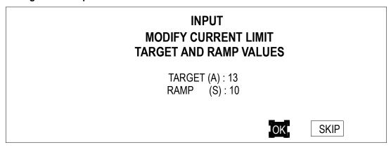
Press SKIP to proceed or OK to change values. If Operator selects SKIP, the Mimic Display screen is momentarily displayed, followed by the screen enabling modification of DC Bus Setpoint.
